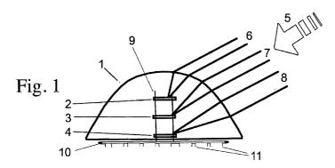
(57) Abstract: For generation of solar energy on limited space, like those on cars and airplanes, a system of multi-staged targets, encapsulated in a parabolic shaped lentil or mirror system is disclosed, wherein impinging light from different directions are directed on a stack of solar converting chips. These are embedded in a heat-transferring optical medium so to avoid overheating, whereas the parabolic capsule may consist of glass or glass -clear plastics, as e.g. polycarbonate copolymers.
